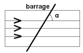
The figure show the setup of a barrage at an angle  $\alpha$  to the current lines. As the current speed increases with both the value of angle diminishes, and the lenght of the barrage go bigger.
